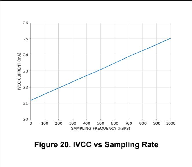
Figure 20. IVCC vs Sampling Rate
