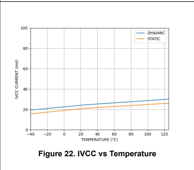
Figure 22. IVCC vs Temperature
