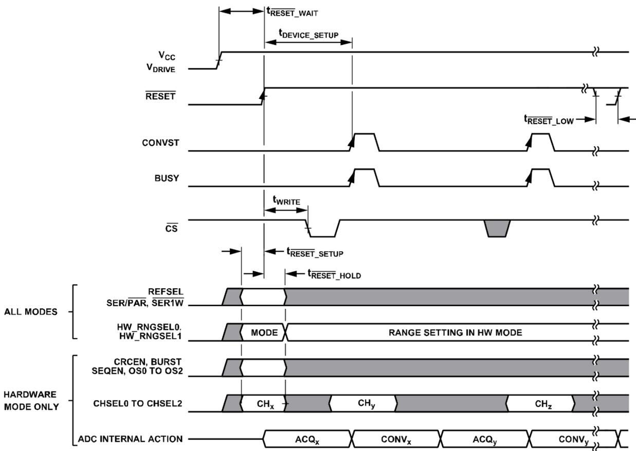
Figure 3. Reset Timing Diagram
