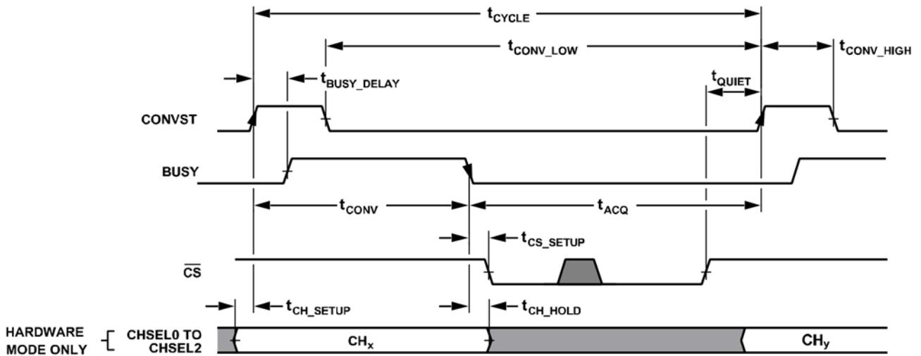
Figure 2. Universal Timing Diagram Across All Interfaces
