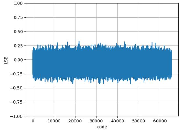
Figure 12. Typical DNL,  $\pm 10\text{V}$  Range
