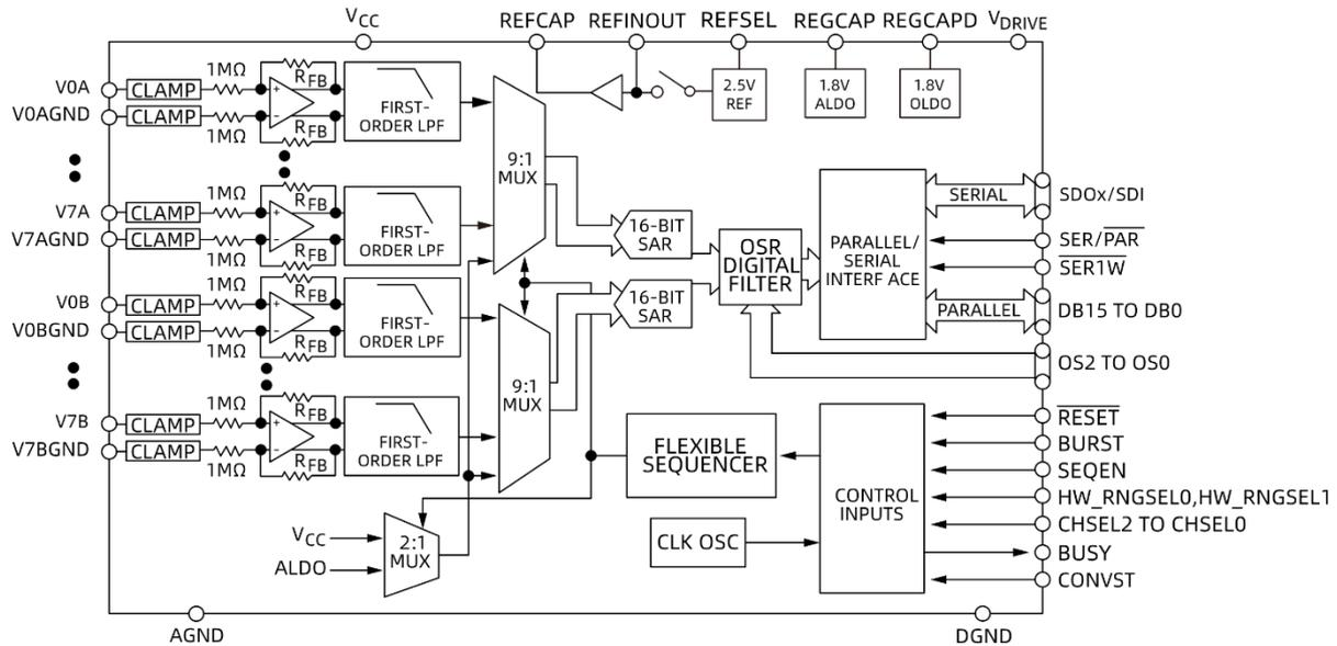
Figure 30. GD30AD33G0 Functional Block Diagram
