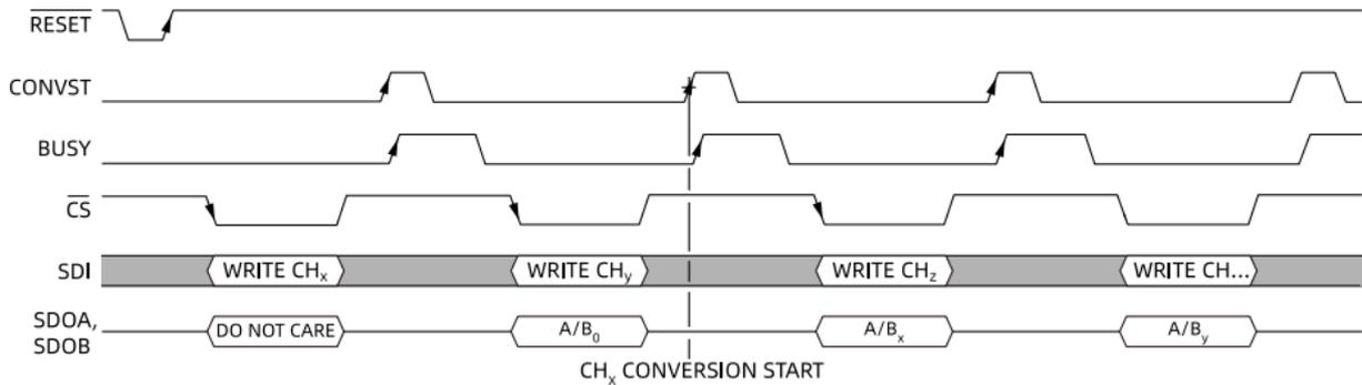
Figure 34. Software Serial Mode Channel Conversion Settings
