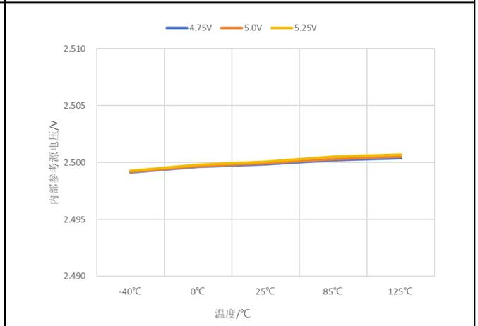
Figure 10. Internal Reference Source Temperature Characteristics
