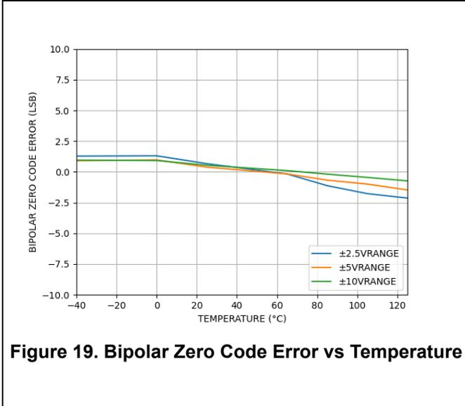
Figure 19. Bipolar Zero Code Error vs Temperature
