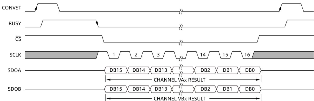
**Figure 39. Serial Interface, 2-Wire Mode**
