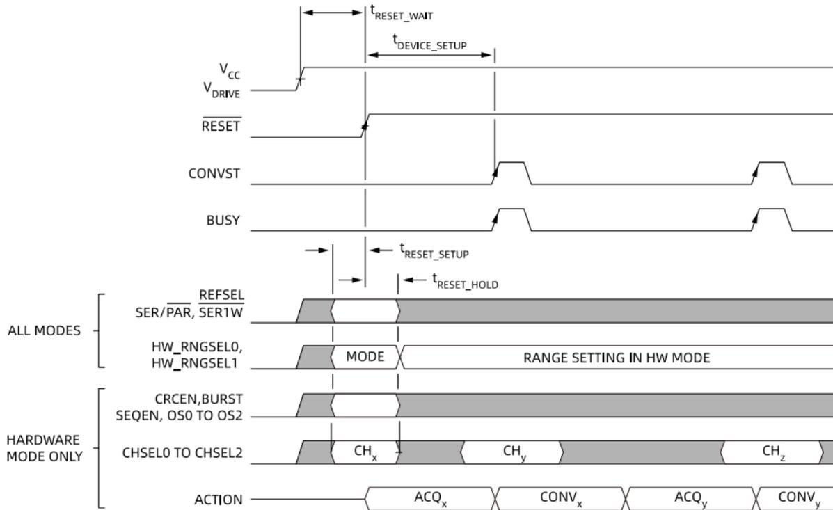
Figure 32. GD30AD33G0 Configuration During Reset
