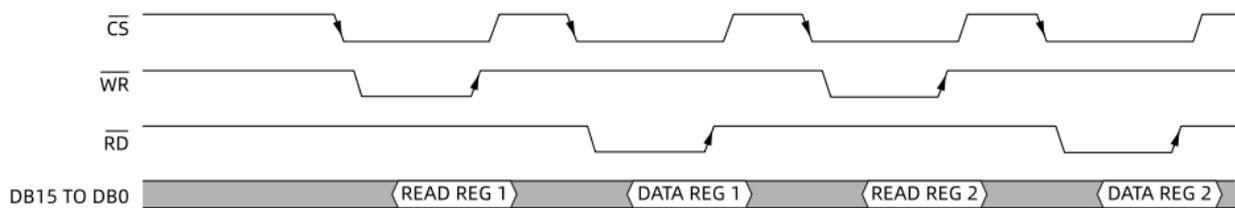
Figure 38. Parallel Interface Register Read Operation
