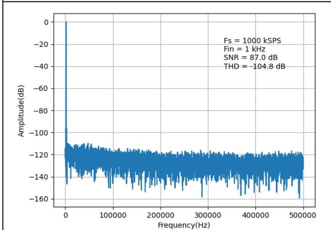
Figure 9. Fast Fourier Transform (FFT),  $\pm 2.5\text{V}$  Range
