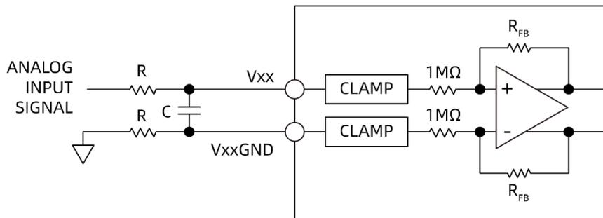
Figure 26. Input Resistance Matching of Analog Inputs
