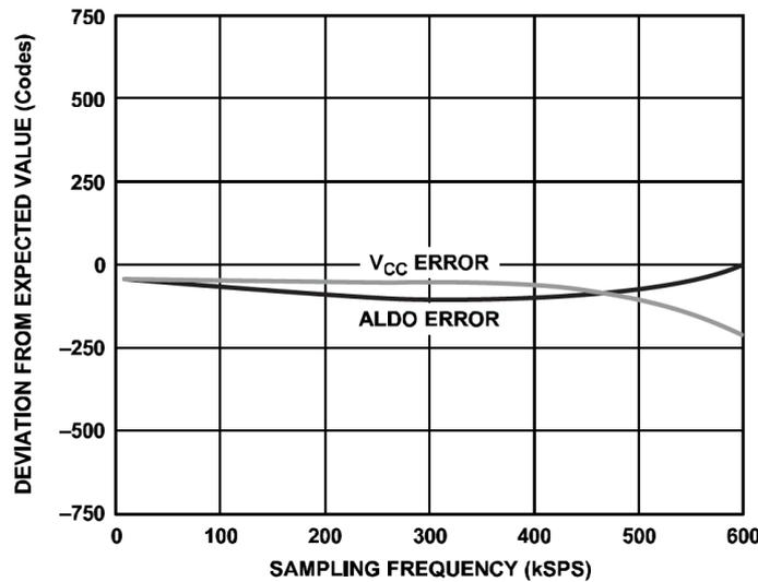
Figure 47. Deviation from Expected Value vs. Sampling Frequency
