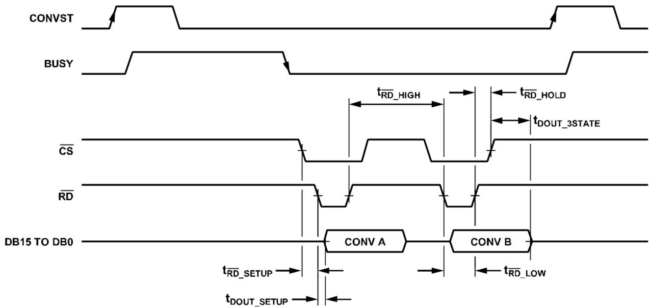
Figure 4. Parallel Read Timing Diagram
