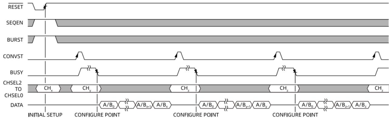
Figure 45. BURST Sequencer Hardware Mode
