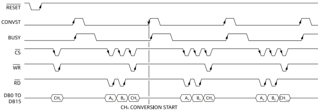
Figure 35. Software Parallel Mode Channel Conversion Settings
