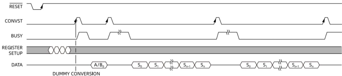
Figure 46. BURST Sequencer Software Mode
