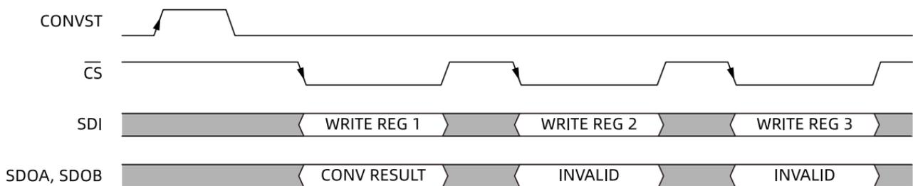
Figure 41. Serial Interface Register Write Operation
