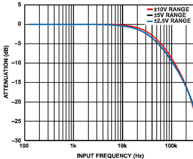
Figure 27. Simulated Anti-Aliasing Filter Frequency Response
