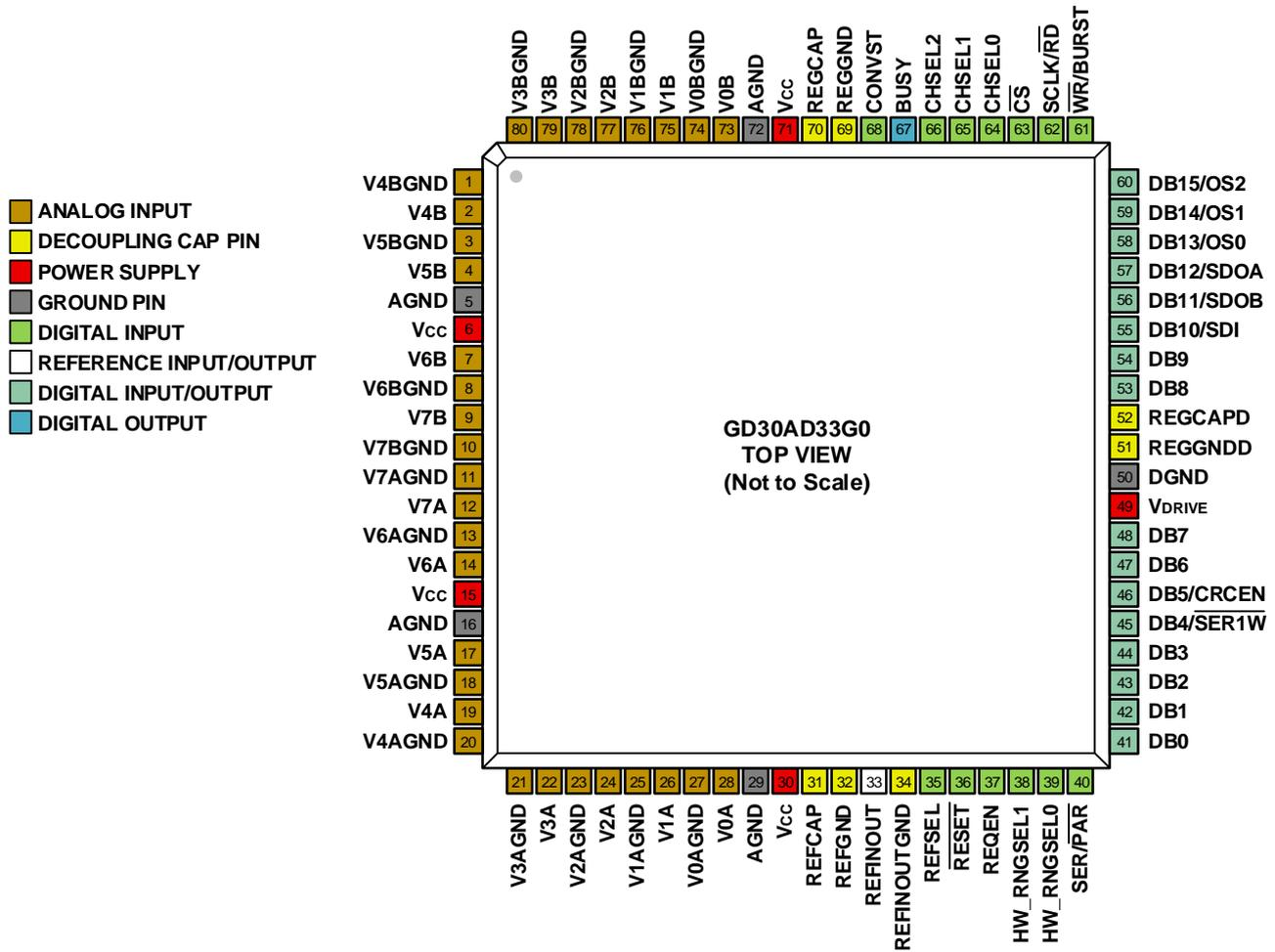
Figure 1. Pin Configuration
