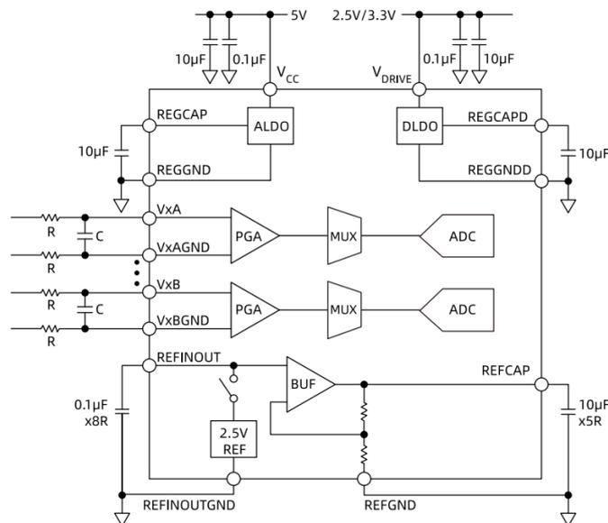
Figure 31. Typical External Connections
