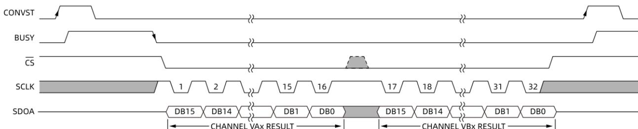
**Figure 40. Serial Interface, 1-Wire Mode**
