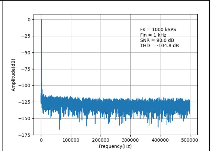
Figure 8. Fast Fourier Transform (FFT),  $\pm 5\text{V}$  Range
