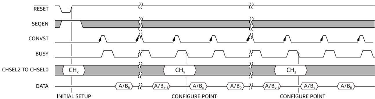
**Figure 43. Hardware Mode Sequencer Configuration**
