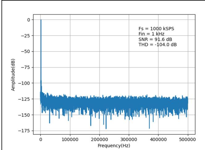
Figure 7. Fast Fourier Transform (FFT),  $\pm 10\text{V}$  Range
